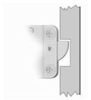
In the **LOCKED** position, there should be approximately 1 mm clearance between the lock bolt and the cavity in the blocking bar of the boltwork. The lock bolt must move freely into the cavity.
